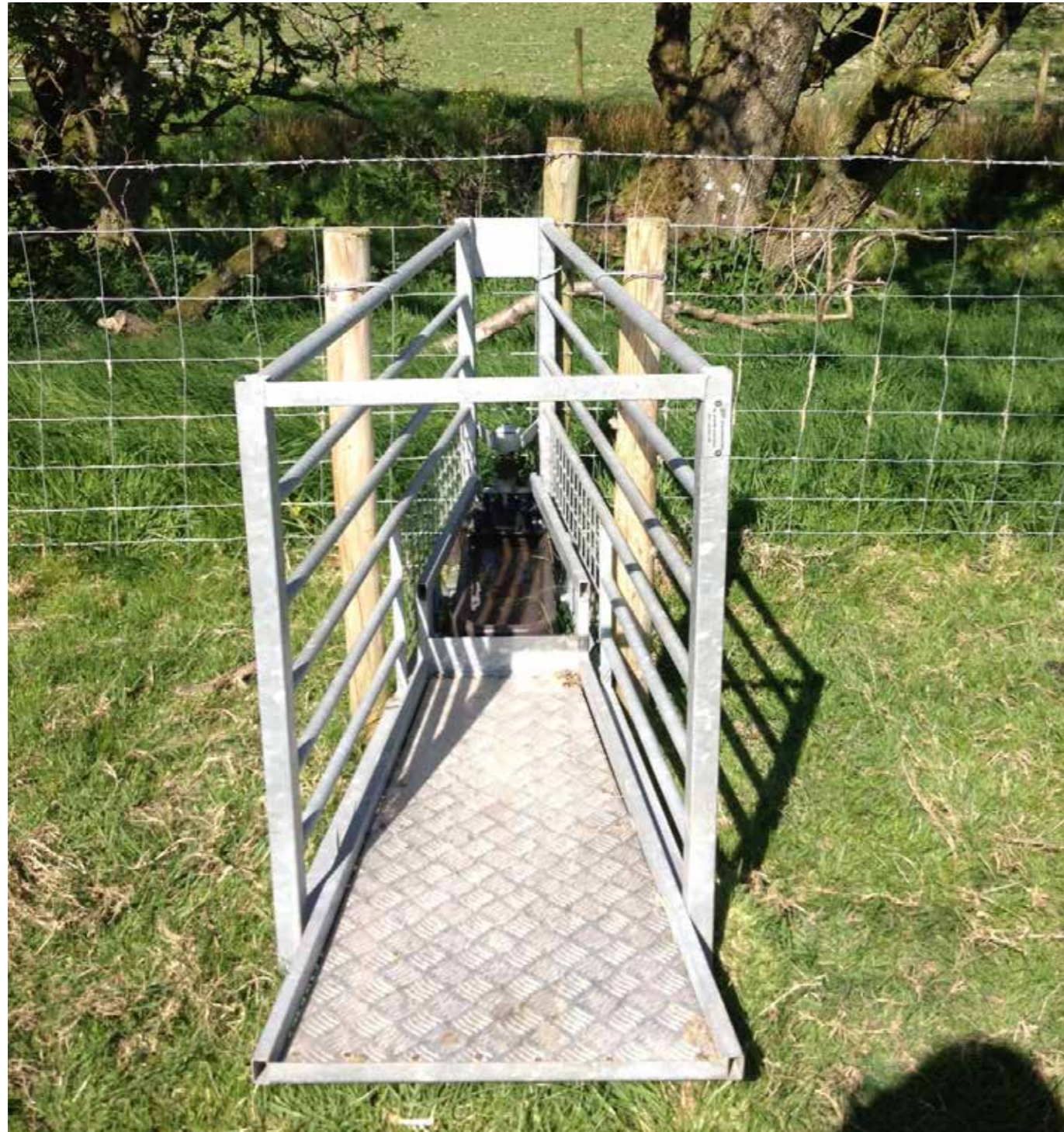
Sheep-operated pasture pump providing water from a fenced-off tributary of the River Ithon in the Wye
