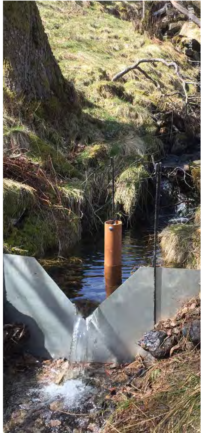
Weir and equipment to measure streamflow in a small upland catchment.
